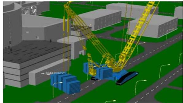
Fig. 9. Dynamic Display of Crawler Crane Counterweight and Reactor Building Distance
