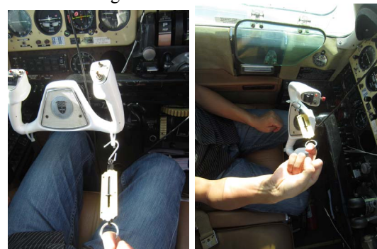
Figure 1. Spring balance used in Baron E55 static stability test
