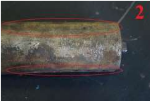
Fig. 1. Rollers wear characteristic at jamming
