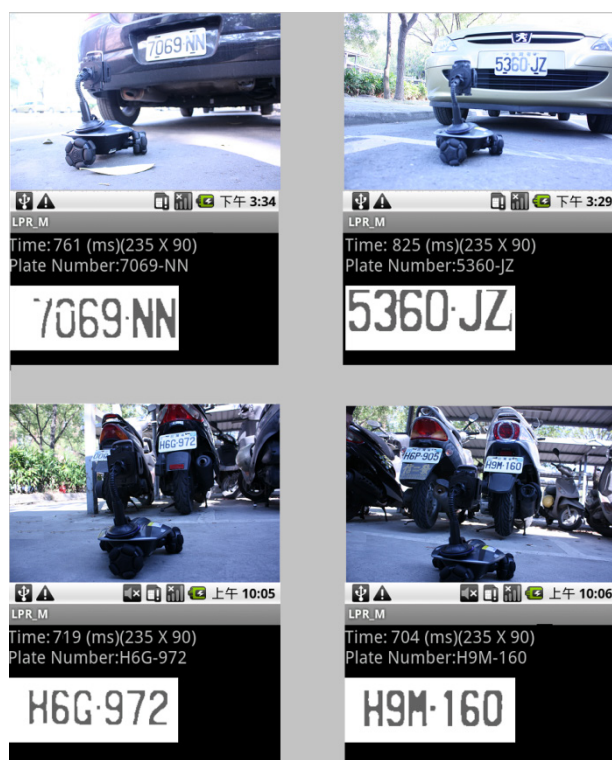
Fig. 4. Field trial about OCR results of the developed Android-based patrol robot featuring AVP and APR.
