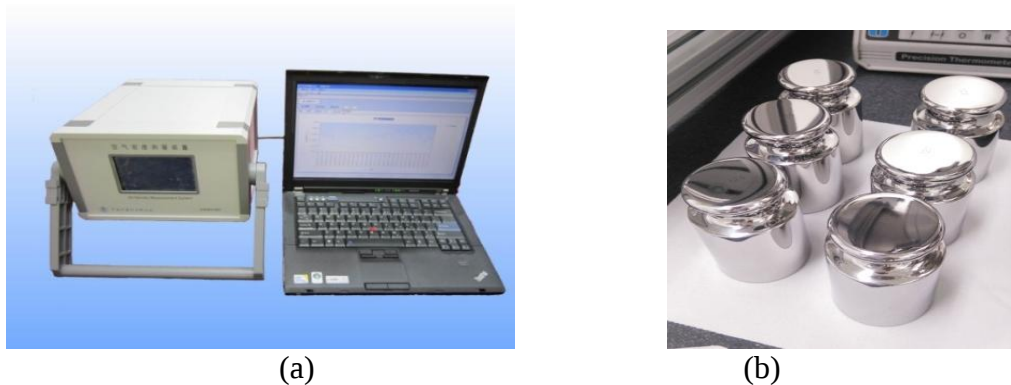
Figure 2. Pictures of air density measurement system (a) and test samples of 1 kg (b)
