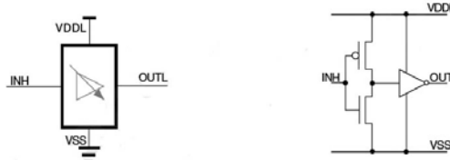
Fig. 2 Conversion from high voltage to low voltage
