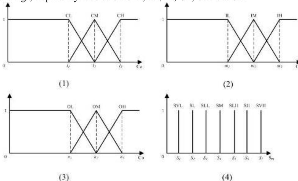
Fig. 3 Membership Functions and Singletons((1)~(3) are Membership Functions in IF Part, (4) is Singletons in THEN Part)
