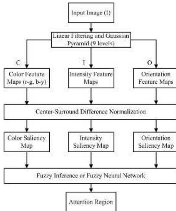
Fig. 1 Overall Procedure for Proposed System
