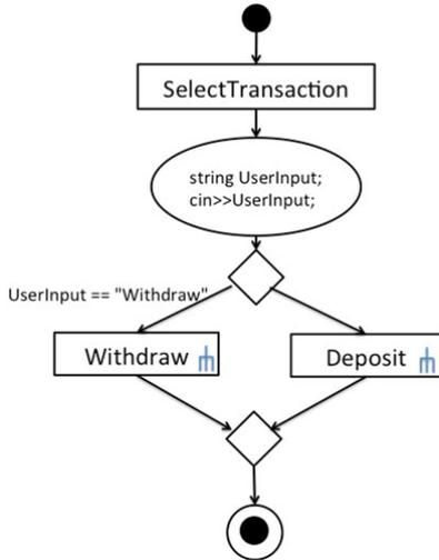
Fig. 5. The Extended Activity Diagram.
