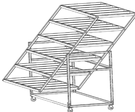
Fig. 6 Design Results of the Sprout Vertical Cultivation Device
