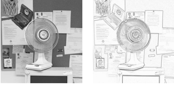
Figure 1: Original image (left) and its fuzzy edge image (right)
