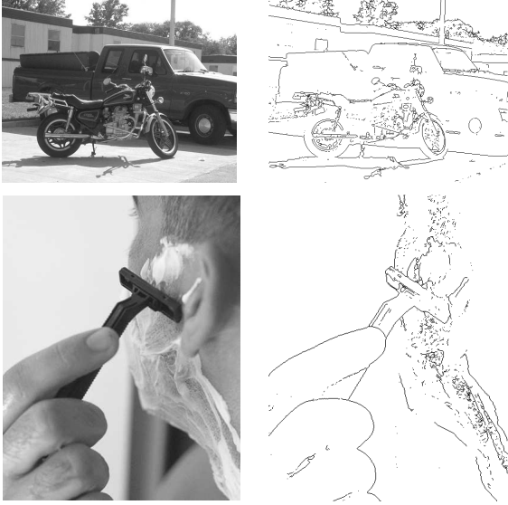
Figure 4: Original image (left) and its binary thin edge image (right) using Algorithm 2 with the Otsu's method.
