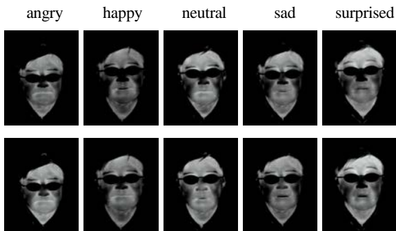
Fig. 3. Thermal face images belonging to major clusters of training data at 0.3 seconds before starting to speak “taro” (upper) and “tsubasa” (lower).
