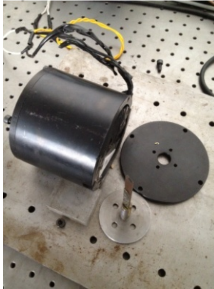
Fig. 5 Improved actuator and its driving structure
