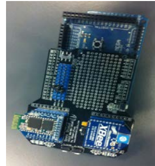
Figure 2. Arduino Uno with beeshielded Bluetooth and Xbee.
