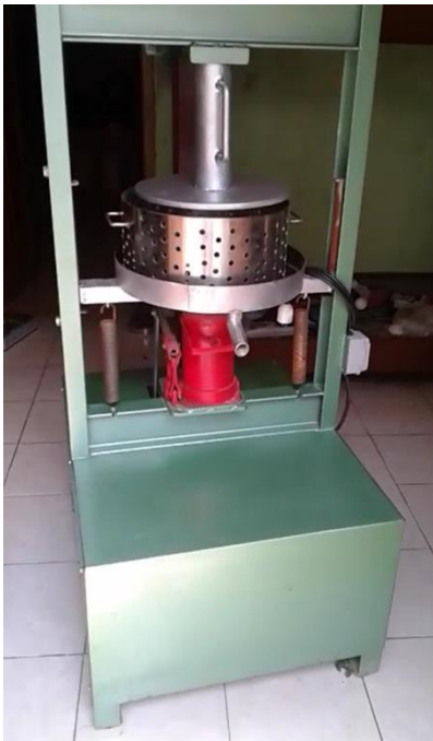
Figure 6. The electrical squeezer machine construction.
