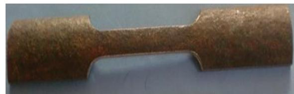
Figure 3. Tensile test specimen tube no 47 [11]
