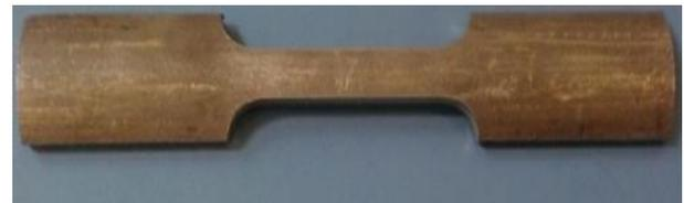
Figure 4. Tensile test specimen replacement tube [11]
