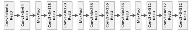
Figure 2 | The first 10 convolution layers of the VGG-16 network. Rectified linear unit (ReLU).
