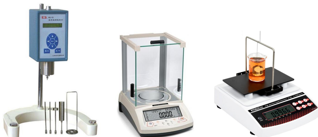
Figure 1 RV20 rotary viscometer, electronic scales and density meter
