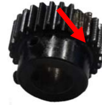
FIGURE III. SEEDED FAULT ON SUN GEAR
