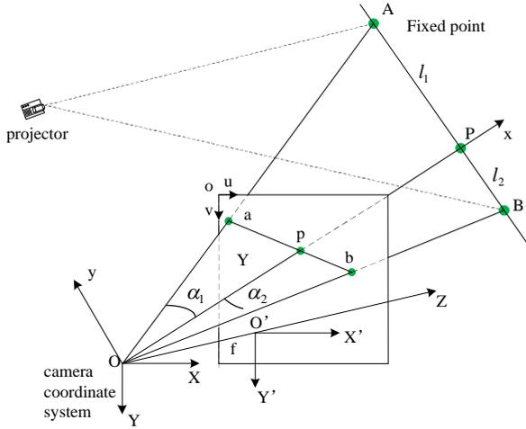
Fig. 2. Linear structured light sensing system calibration diagram
