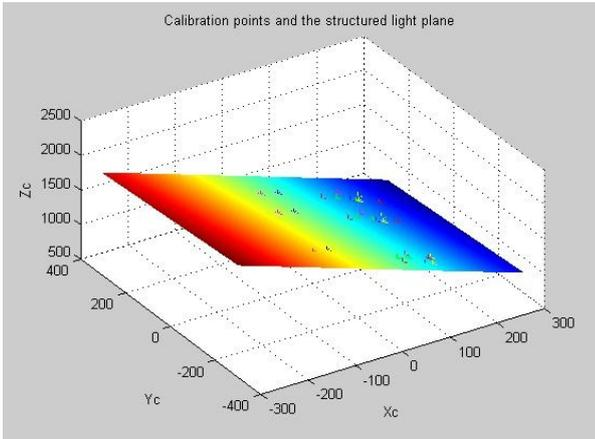
Fig. 5. The calibration points and the light plane in the camera coordinate system
