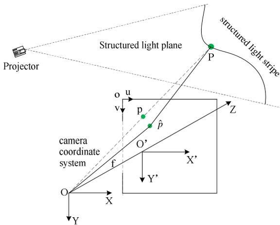
Fig. 1. Geometric model of linear structured light active vision sensing system
