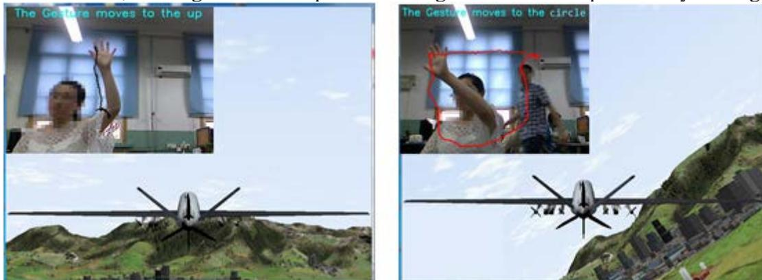
Fig.8 UAV flight controlled by dynamic gestures
